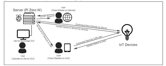
With this design, even if the server's processing power is low, it can still support a number of users from LAN connection as the more client is connected to the system, there are more devices to share the processing load in controlling all devices.
